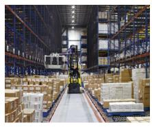
The racking systems utilize the 40' height clearance of the warehouse and innovations in racking technology to optimize storage capacity – using 2, 3 and 4 deep push back systems.
